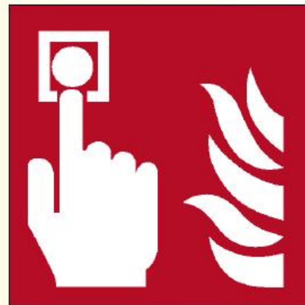
Fire alarm call point
