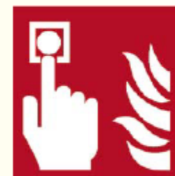
Fire alarm call point
